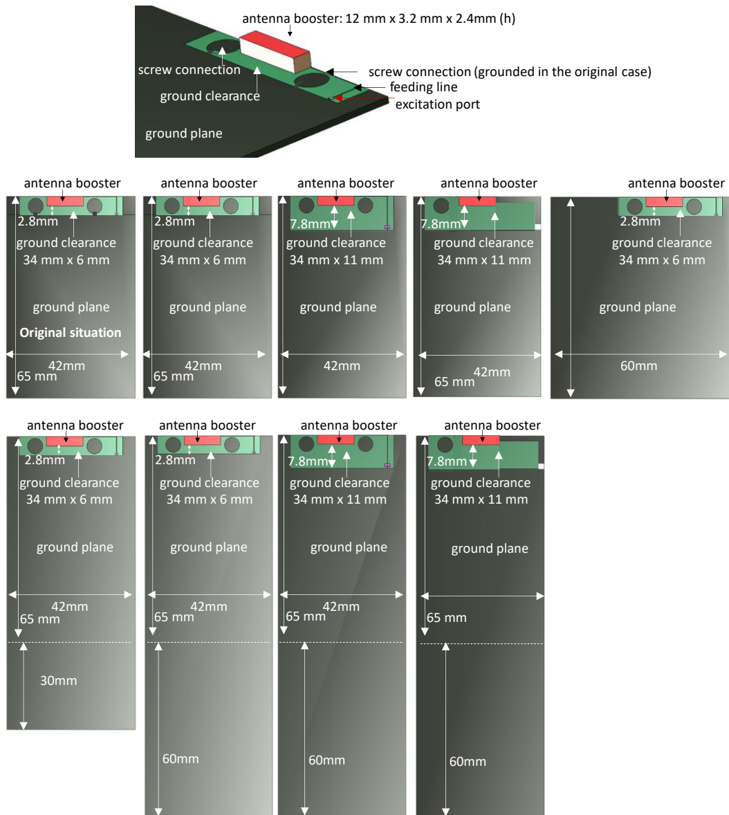
Figure 1 - Cases considered in the analysis: screw connectors, change ground clearance, change feeding location, and change PCB size. Each scenario has a matching network at the excitation port which comprises lumped elements (capacitors and inductors). Only the original case has the screw connectors connected to the ground of the PCB; at the other cases, such screw connectors are floating (non-grounded).
