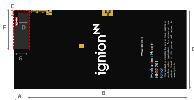
Figure 4 – EB_NN02-201-2G/3G-USA evaluation board providing operation at 2G/3G-USA band (824 – 894 MHz and 1850 – 2170 MHz).
