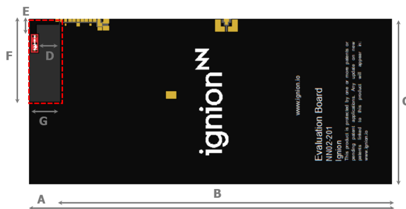
Figure 1 – EB_NN02-201-2G_3G-Europe. Evaluation board providing operation at 2G/3G-Europe band (880 – 960 MHz and 1710 – 2170 MHz).
