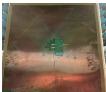
Figure 12 – Set-ups analyzed considering the presence of metal, 10mm of distance between the PCB and metal and two different positions: PCB located in the middle and PCB located on the corner.
